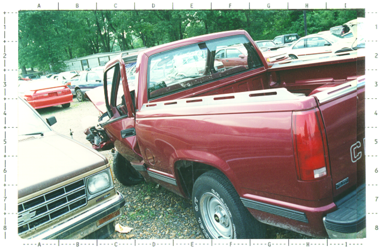
# 71 -- Left back view of 1988 Chevrolet C-1500 pickup; NOTE: outward bowing to left front (driver's) door & induced cargo bed damage
